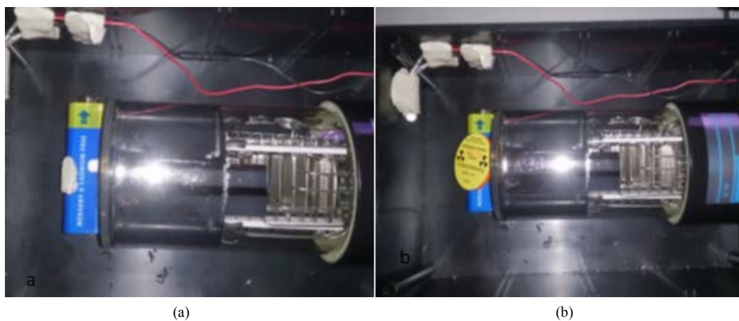
Figure 3. (a) Scintillation crystal coupled to Hamamatsu photomultiplier tube (R878); (b) Gamma source mounted upon the crystal.
