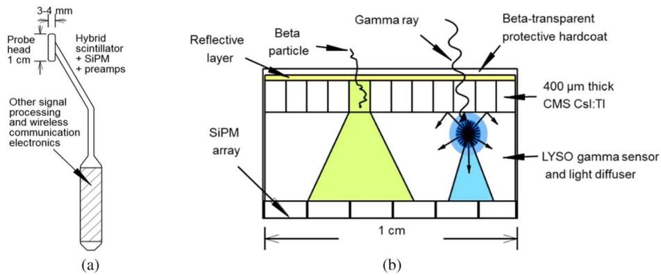
Fig. 1. (a) Conceptual design of the imaging probe head. (b) The ultimate probe design which realizes a wireless handheld unit.
