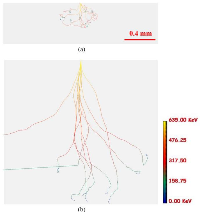
Fig. 2. Range of F-18 positrons in CsI:Tl (a) and water (b). For clarity, we only show trajectories of 10 electrons at 635 keV. We utilized CASINO simulation software available at [25].
