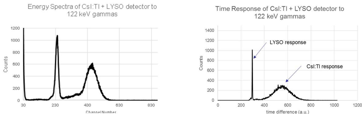
Fig. 5. Energy and time spectra of the hybrid scintillator exposed to 122 keV gammas. Due to the longer decay time of the CsI:Tl, one can reject the LYSO signal using PSD.
