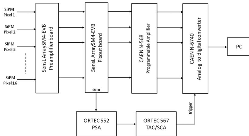
Fig. 3. Data acquisition setup for generating 2D position histogram, 1D line profiles and energy spectra. Note that pulse shape discrimination is implemented using ORTEC 552 PSA and 567 TAC/SCA units. This allows to trigger the ADC unit when the signal is originating from CsI:Tl scintillator.
