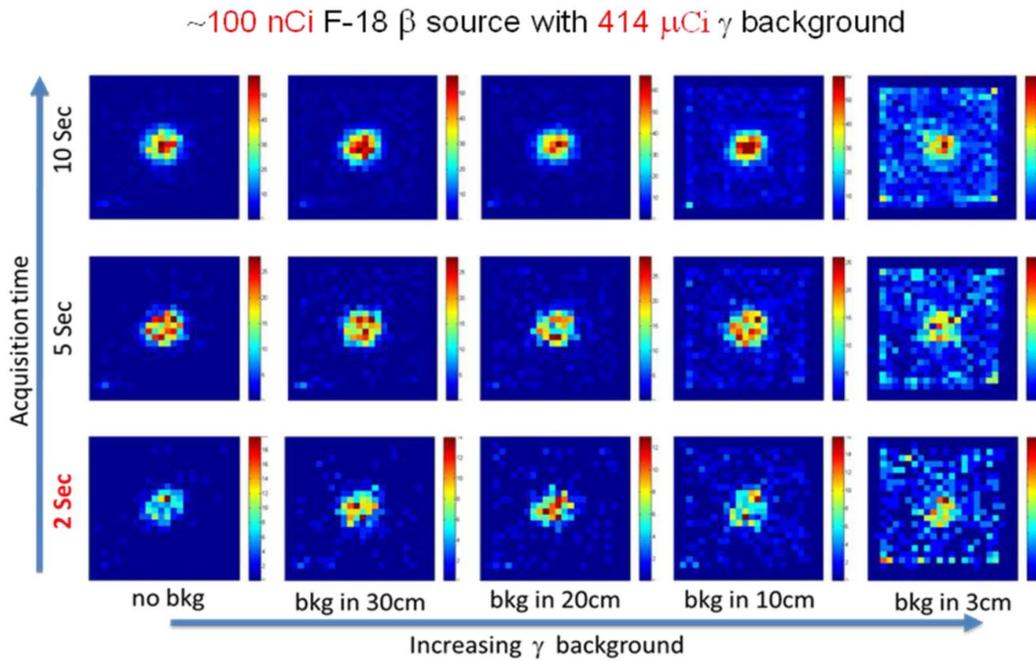
Fig. 8. Acquisition time versus increasing gamma background strength. No smoothing or baseline correction was applied to the results. The data show that the probe can comfortably detect beta signal with 10 second acquisition time at all background distance. However, SNR and the quality of the image reduce dramatically with short acquisition times (e.g. 2 seconds) and short background-detector distances.
