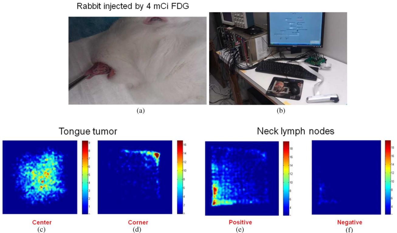
Fig. 10. (a) The rabbit with tongue tumor. Tumor cells were injected to the animal's tongue two weeks before the experiment. (b) photo of the probe with associated electronics and display. (c) and (d) show images of the tongue tumor and how the probe can be used to locate the tumor margin. (e) and (f) show images of the positive and negative lymph nodes in rabbit's neck. The results suggest that the probe can be used to check the status of the lymph nodes ex-vivo.
