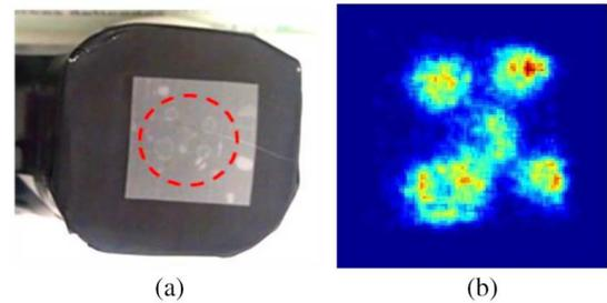
Fig. 9. (a) five F-18 drops, with total activity of  $\sim 10$  nCi placed on Scotch tape. (b) acquired image of the drops showing that the probe can detect weak beta signals.
