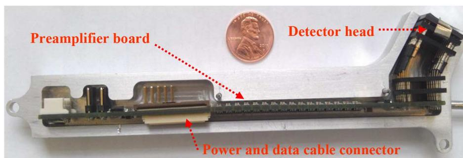
Fig. 6. Photo of the prototype probe consisting of detector head, PreAmp board, and aluminum housing.
