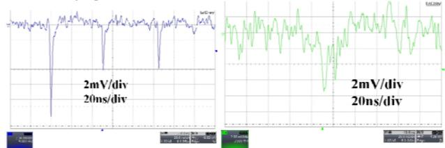
Fig.10. White electronic noise and dark counts on fast output of single pixel (left) and block (right).
