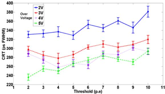
Fig.7. CRT as a function of the LED threshold for different bias voltages.
