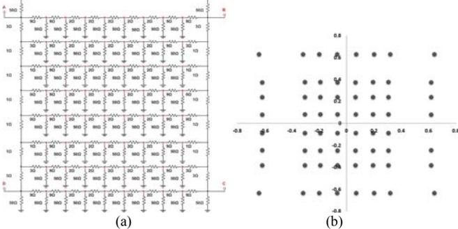
Fig.4. (a) Schematic of resistor network (b) Position map of 64 channels
