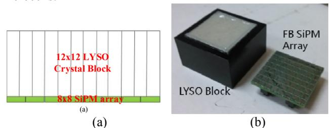
Fig.1. (a) Side view of detector module (b) Photographic image of LYSO block and FB SiPM array.
