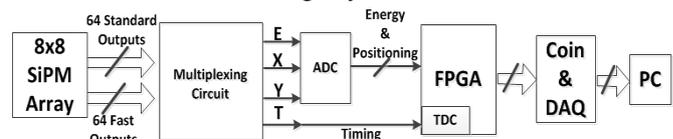
Fig.2. Block diagram of readout architecture.
