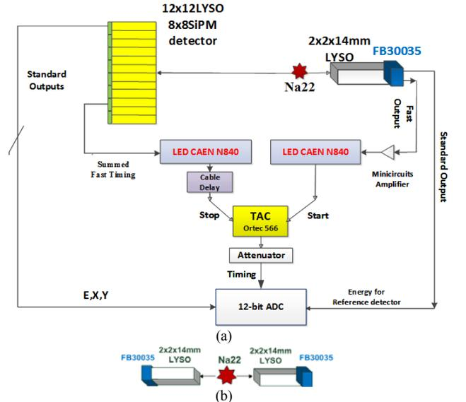
Fig.5. (a) Coincidence measurement setup for detector module (b) Single pixel timing resolution measurement
