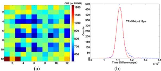
Fig.8. (a) CRT across the 12 x 12 crystal block; (b) Best timing spectrum
