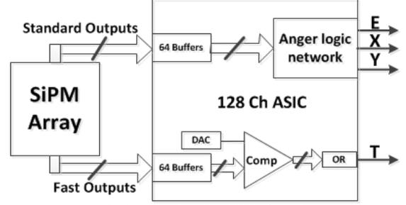
Fig.4. ASIC based multiplexing scheme
