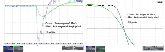
Fig.9. Typical waveform(left) and initial rising edge(right) of fast output of block and single pixel.
