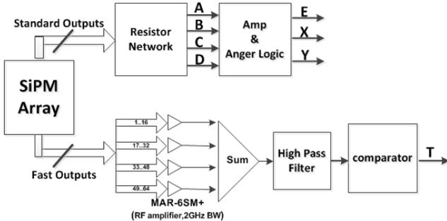
Fig.3. Conventional electronics based multiplexing scheme
