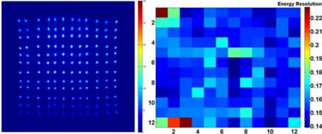
Fig.6. (a) Flood histogram of the crystal block. (b)Energy resolution across all crystals of the block
