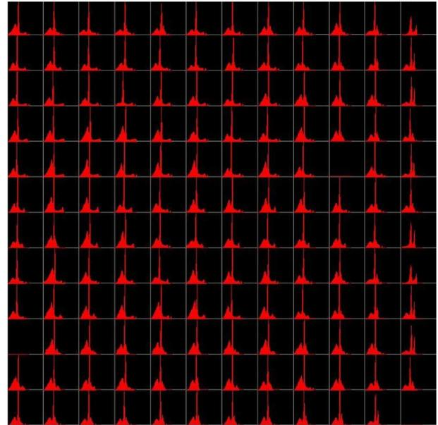
Fig. 11. Measured energy spectra of 144 channels in one detector module.
