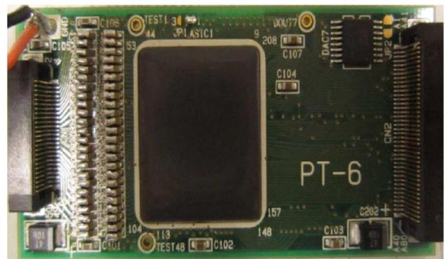
Fig. 6. Front-end ASIC board for the gamma detector.
