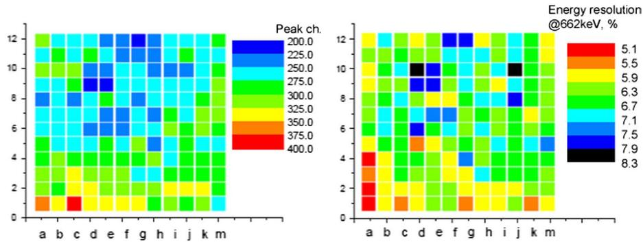
Fig. 3. The variation of energy resolution and signal amplitude in the APD-Ce:GAGG matrix for the  $^{137}\text{Cs}$  source.
