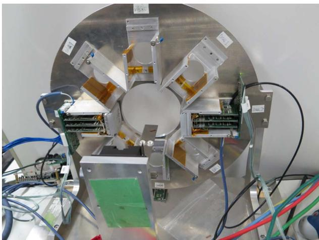
Fig. 10. The PET system with two detector modules.
