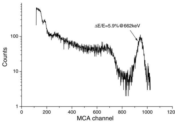
Fig. 4. Example of an energy spectrum obtained with a single pixel in the APD-Ce:GAGG matrix for the  $^{137}\text{Cs}$  source.
