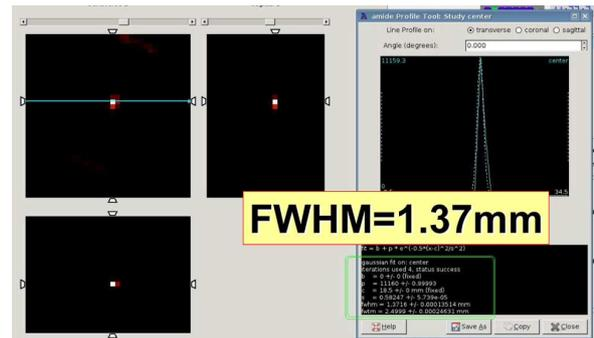
Fig. 12. Reconstructed image of a point source of  $^{22}\text{Na}$ .
