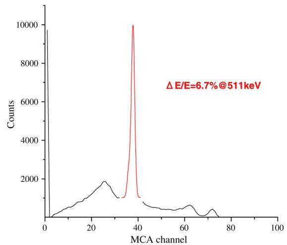
Fig. 7. Energy resolution for 511 keV gamma rays from  $\text{Na}^{22}$  source measured with ToT output by Altera Cyclone III FPGA.
