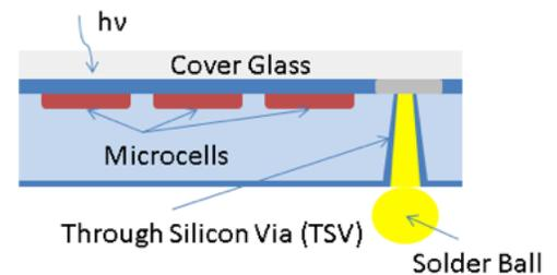
Figure 1, The SensL TSV sensor (top) and the TSV concept (bottom).
