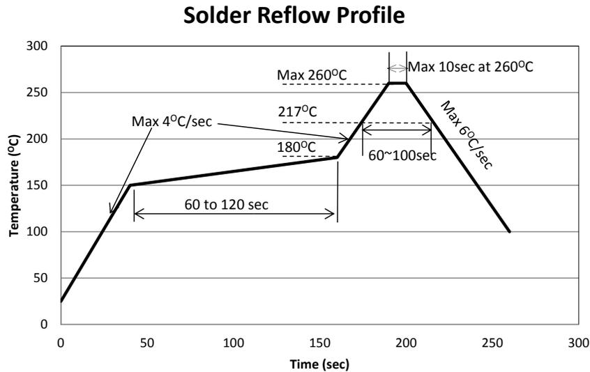
Figure 2, Solder reflow profile
